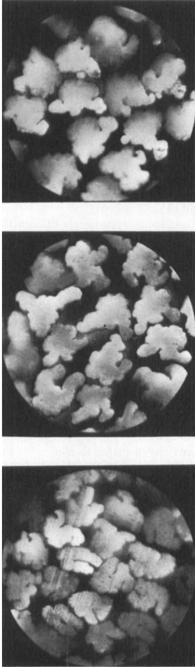
FIG. 1. The effect of graft modification of viscose fibers on cross-sectional area. Left: Crimped rayon staple, with a denier of 8.74 and a ratio of 1; and with a relative cross-sectional area of 143 and a ratio of 1. Center: Grafted with a phosphorous-containing polyvinyl compound (46%), with a denier of 12.9 and a ratio of 1.47; and with a relative cross-sectional area of 204 and a ratio of 1.43. Right: Grafted with acrylonitrile (45%), with a denier of 12.7 and a ratio of 1.45; and with a relative cross-sectional area of 212 and a ratio of 1.48.
